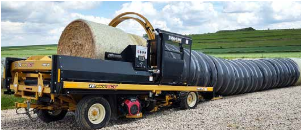
Figure 1. Dry alfalfa bales wrapped in breathable film using the modified bale wrapper. Note spiral wrap of tape at the training edge seam to seal the film.
